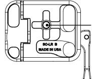
Center hole is keyed with a double "tongue-and-groove" to allow for multidirection mounting options. Threaded 3/8"-16 hole.
