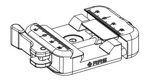
Really Right Stuff SOAR lever-release clamps use our patent pending dual clamp design to attach to the RRS 1.5" dovetail standard and Picatinny rail sections.
